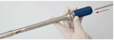
Insert CS 2256-22 into the instrument through CS 2256-01. Ensure that CS 2256-22 remains freely movable.
